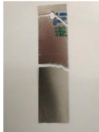
Mo plate with Nb coating after testing
